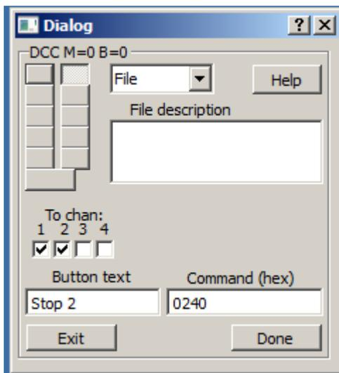
Thus when button 2 is pressed (the button with text “Stop 2”) the command sequence 0x02 0x40 is send to the Gertbot. There it will be replicated to go out on channels 1 *and* 2. The Gertbot will also add the checksum byte (which will be 0x42).
