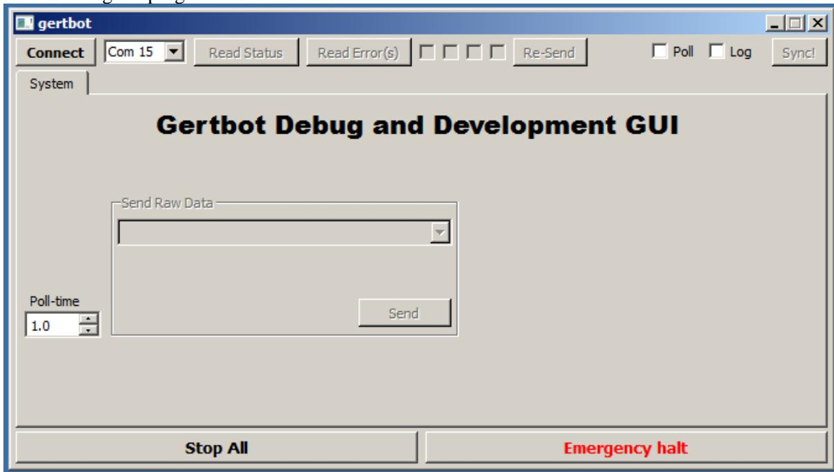
When you press the 'connect' button the program will look for any connected boards and change its appearance accordingly.
